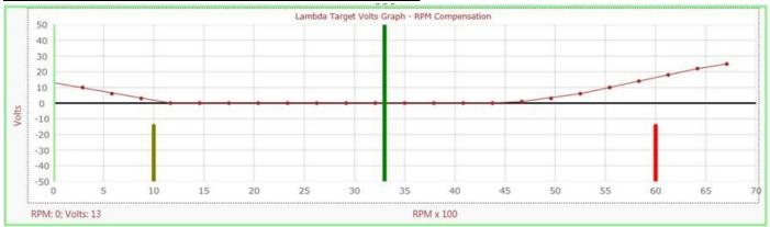
This graph will adjust compensation in the RPM range. Outside the 2 limits will be no control.
